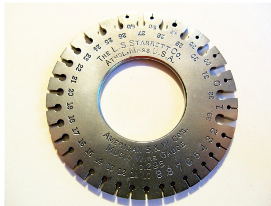
Figure 1. Device for measuring wire gauge
