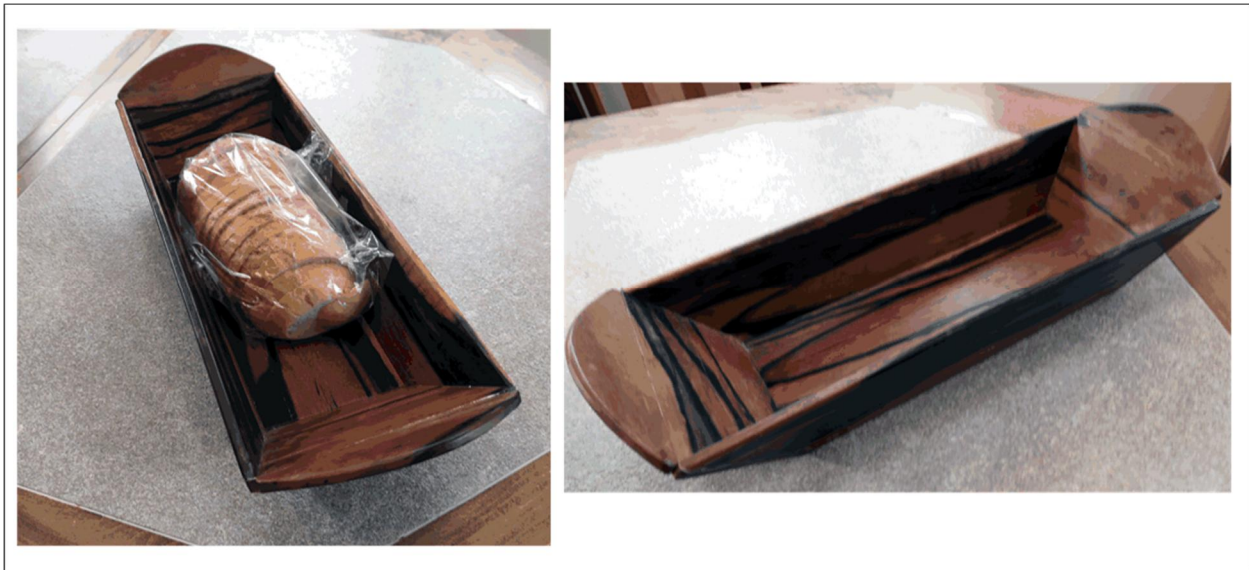
Figure 4. Mario Petrilli's bread-holder project. Long sides slope at 70 degrees from horizontal, and the ends slope at 50 degrees.
