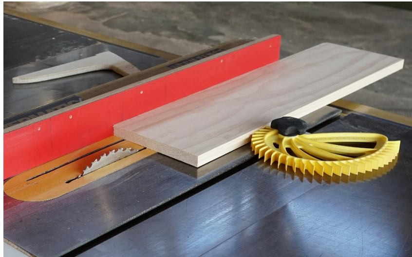
Figure 12. The Hedgehog featherboard is shaped as a Bernoulli spiral.
