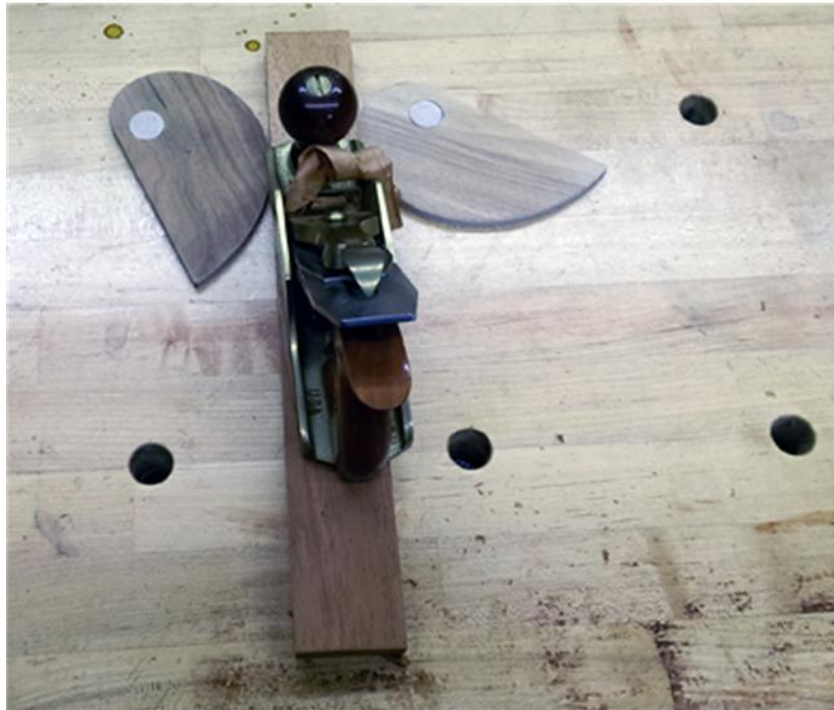
Figure 9. Bernoulli cam clamps in use with a hand plane
