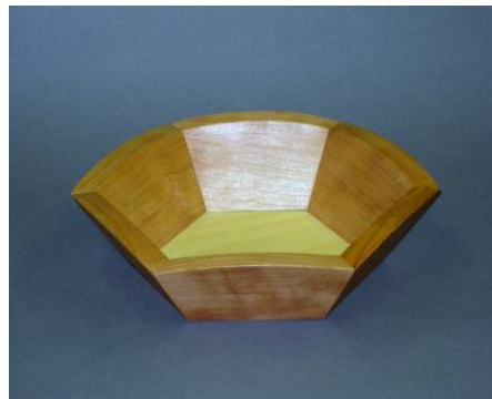
Figure 3. Hexagonal bowl involving compound-angle joinery. Each of the six sides slope outward at 60^\circ from the base.
