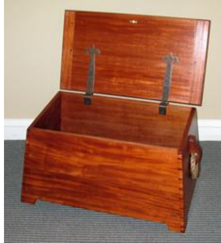
Figure 4. Four sided sea chest having sides that slope inward at 82^\circ from the base.
