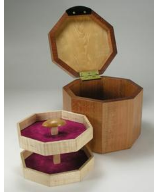
Figure 1. Octagonal jewelry box with removable shelf insert. Made by Vic Barr using maple and cherry woods. The eight sides are at 90^\circ to the base.
