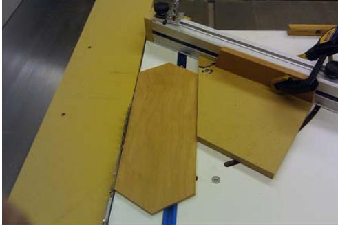
Setting Fence Stop For Remaining Cuts Using Stock
