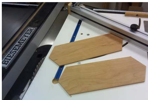
Result of First and Second Cuts On Both Ends Of All Stock
