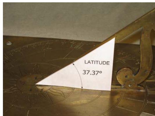
Figure 3. Shows correct hour-line angle for 9:00 a.m. A repair resulted in the gnomon being offset from the dial center and at an incorrect angle.
