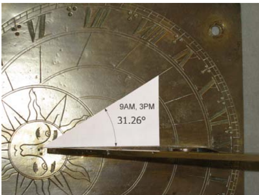
Figure 3. Shows correct hour-line angle for 9:00 a.m. A repair resulted in the gnomon being offset from the dial center and at an incorrect angle.
